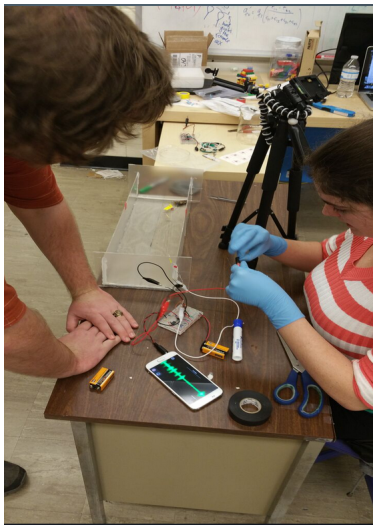
Figure 4: The experimental setup. The complete experimental setup included the arena (pictured on the left), an electronic circuit connecting electrode signals to a cellular phone, the cellular phone running Backyard Brains app, and a tripod positioned above the arena so that the experiments may be filmed.
