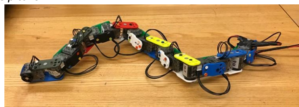
Figure 1: 13-DoF snake robot capable of lateral and vertical bending.
