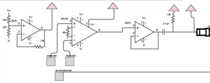
The first op-amp group forms the voltage divider which outputs a 4.5V virtual ground. The second op-amp group forms the gain circuit. The final op-amp group is a low-pass filter that protects the smartphone from a surge (you can calculate the cutoff frequency from the RC-constant).
