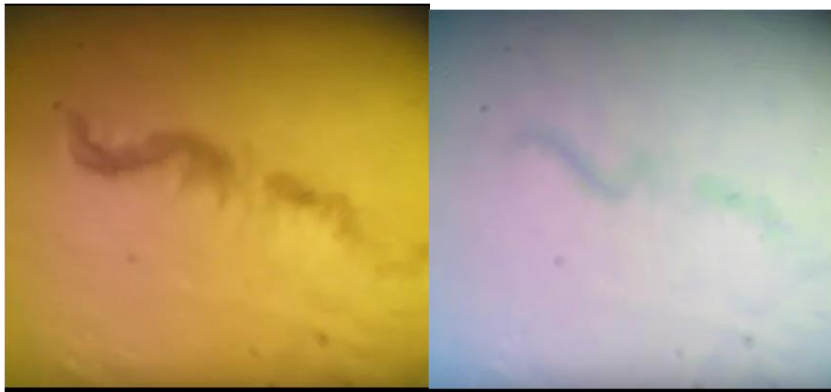
Figure 4. Undulating C. Elegans visualized without and with blue LED excitation light.
